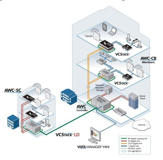
Allied Telesis Autonomous Wave Control (AWC) offers solutions for two of the most common problems with Wireless LANs: initial setup complexity, and on-going performance degradation. Initial WLAN set-up usually requires a site survey to achieve the best coverage, and performance of WLANs can often change over time as external sources of radio interference reduce coverage and bandwidth. These issues can be time-consuming to identify and resolve.
