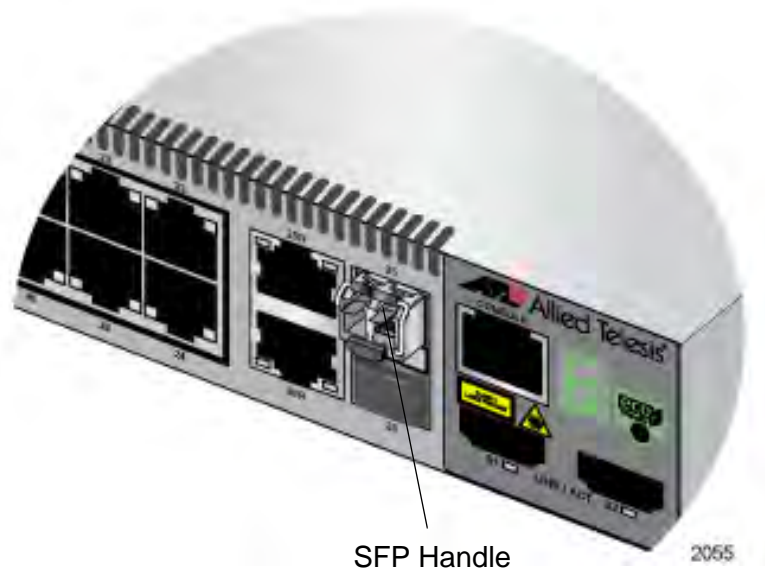
Figure 32. Positioning the SFP Handle in the Upright Position
