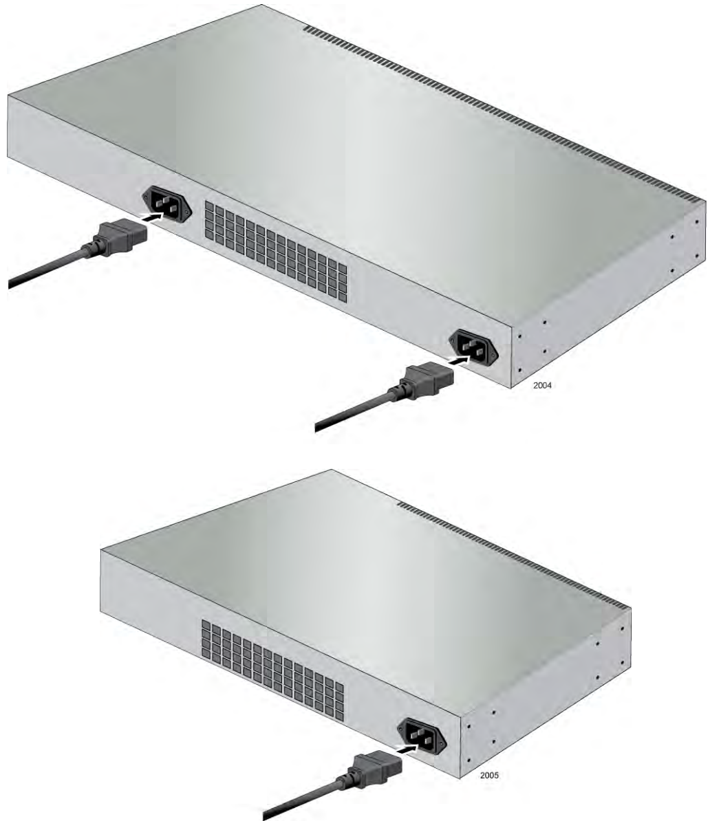
Figure 34. Plugging in the AC Power Cord
