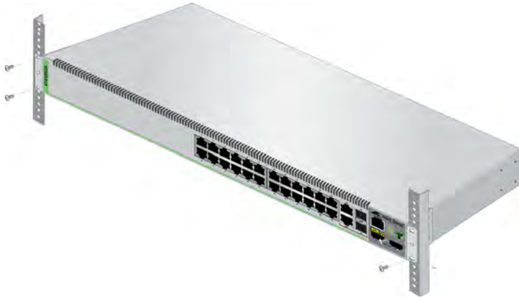
Figure 28. Mounting the Switch in an Equipment Rack
