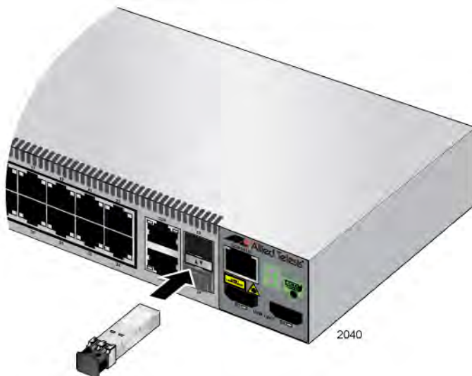
Figure 30. Installing an SFP Transceiver
