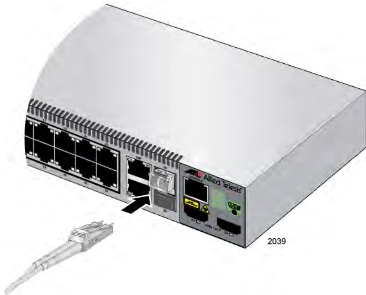
Figure 33. Connecting the Fiber Optic Cable to the SFP Module
