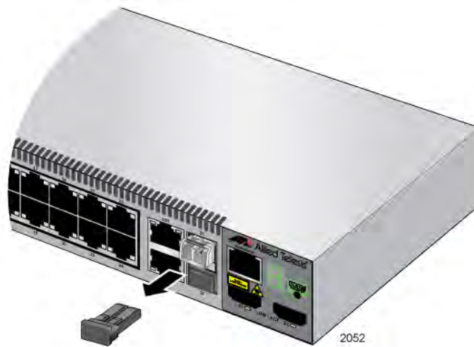
Figure 31. Removing the Dust Cover from the SFP Module
