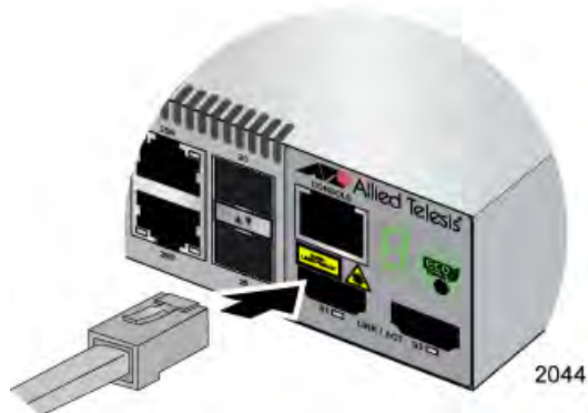
Figure 40. Connecting the Management Cable to the Console Port
