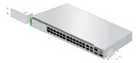
Figure 25. Attaching the Brackets to the AT-8100S/24C Switch to Install the Switch in an Equipment Rack
