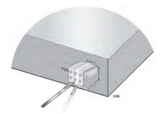
Figure 43. Inserting Wires into the DC Terminal Block
