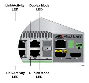
Figure 11. 10/100/1000Base-T Port LEDs
