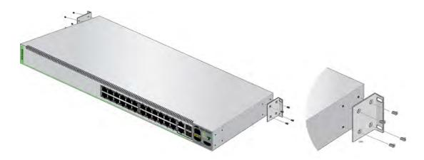
Figure 24. Attaching the Brackets to Install the Switch in an Equipment Rack (Continued)
