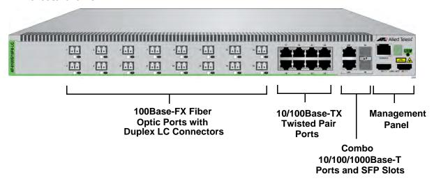
Figure 3. Front Panels of the 8100S Fiber Optic Series
