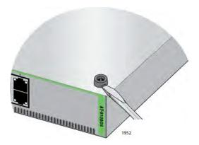
Figure 22. Removing the Rubber Feet
