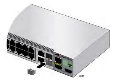
Figure 56. Installing the Dust Cover in the SFP Slot
