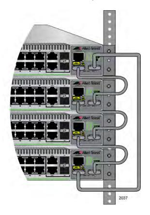
Figure 36. Example Stack of Four Switches with a Redundant Path
