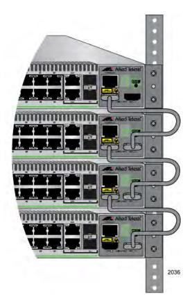
Figure 35. Example Stack of Four Switches
