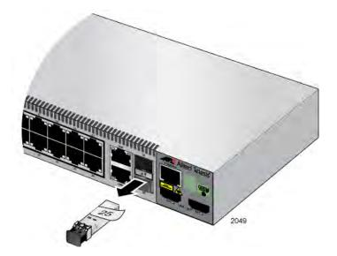
Figure 55. Removing the SFP Module
