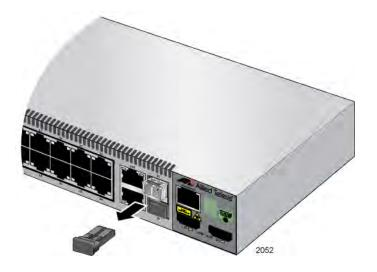
Figure 47. Removing the Dust Cover from the SFP Module
