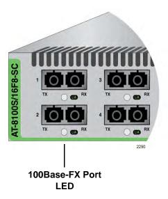
Figure 12. 100Base-FX Port LED
