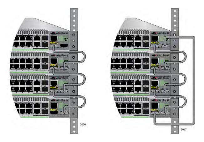
Figure 16 Duplex-chain and Duplex-ring Configurations
