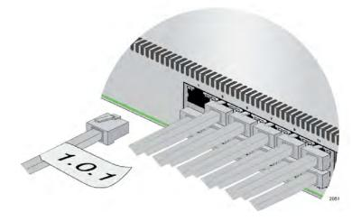
Figure 52. Removing the Network Cables
