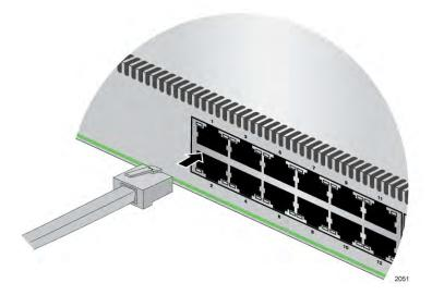
Figure 31. Connecting the Twisted Pair Cable to a Networking Port on the Switch
