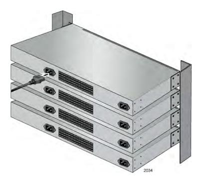
Figure 29. Connecting the AC Power Cord
