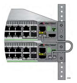
Figure 34. Connecting the Stacking Cable
