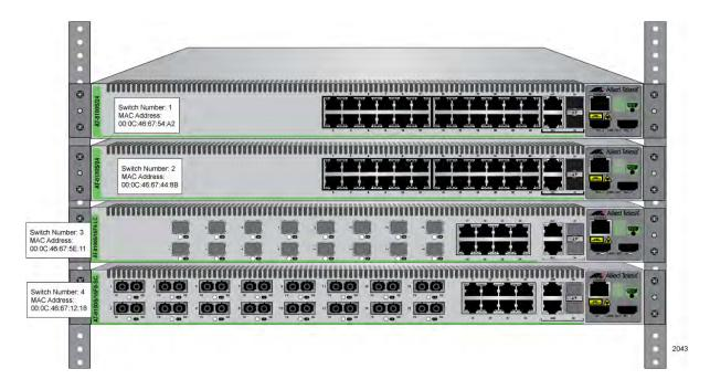
Figure 28. Labelling the Switches
