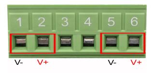
1. Insert AC or DC power wires into the contacts I and 2 for power I, or 5 and 6 for power.
