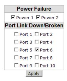
Fault Relay Alarm interface
