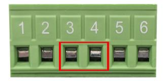
Insert the wires into the fault alarm contacts
