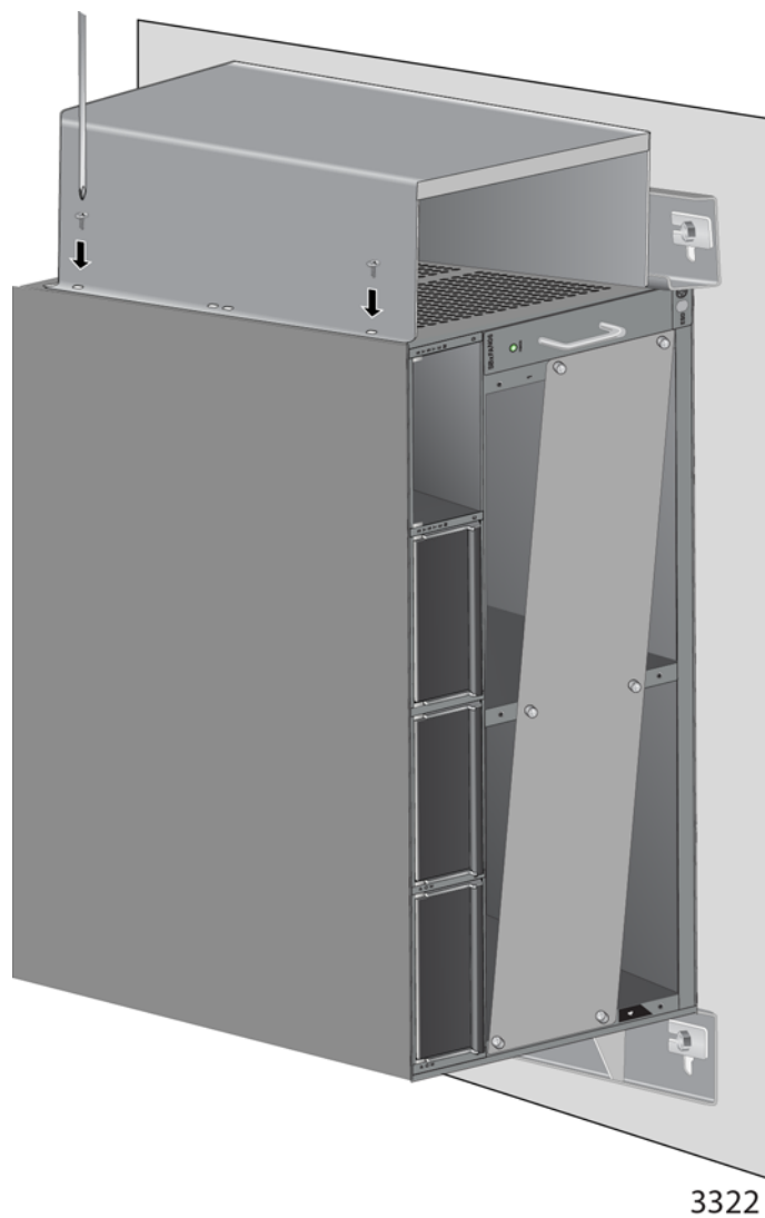
Figure 22. Securing the Top Vent Cover
