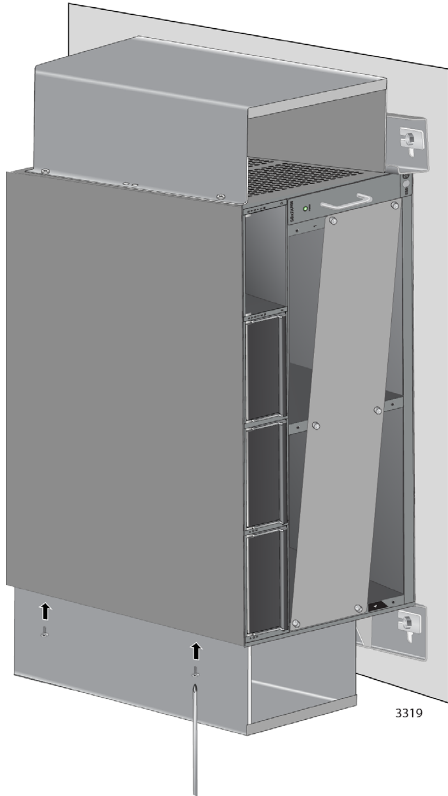
Figure 24. Securing the Bottom Vent Cover
