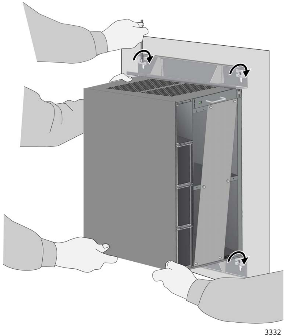
Figure 20. Tightening the Screws
