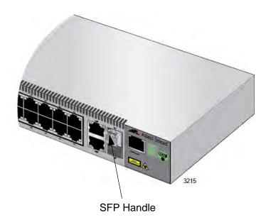
Figure 31. Positioning the SFP Handle in the Upright Position
