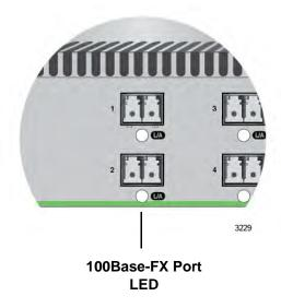
Figure 15. 100Base-FX Port LED
