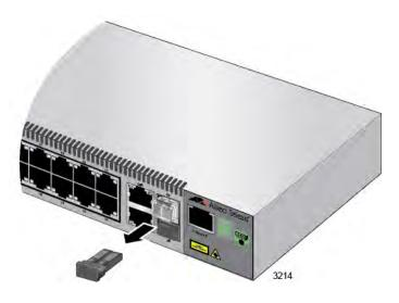
Figure 30. Removing the Dust Cover from the SFP Module
