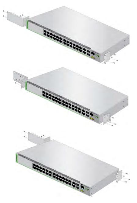
Figure 25. Attaching the Equipment Rack Brackets
