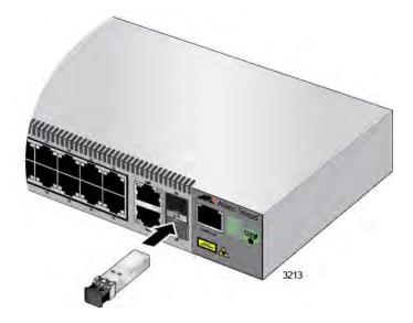
Figure 29. Installing an SFP Transceiver
