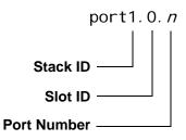
Figure 39. PORT Parameter in the Command Line Interface
