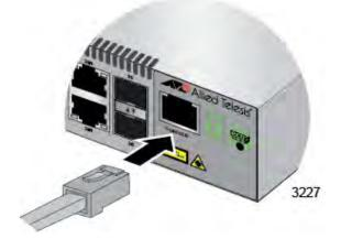
Figure 37. Connecting the Management Cable to the Console Port
