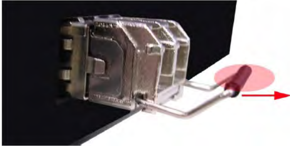
FIGURE 5-5 Pull out the SFP module
