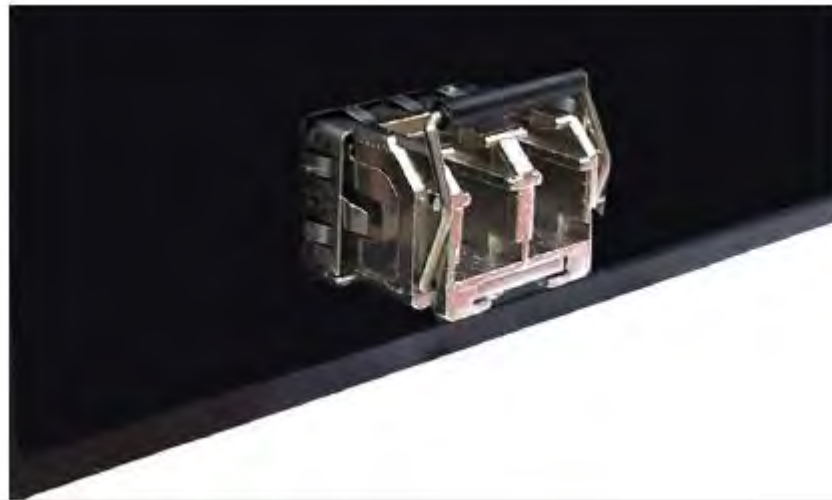
FIGURE 5-2 SFP module inserted into its bay
