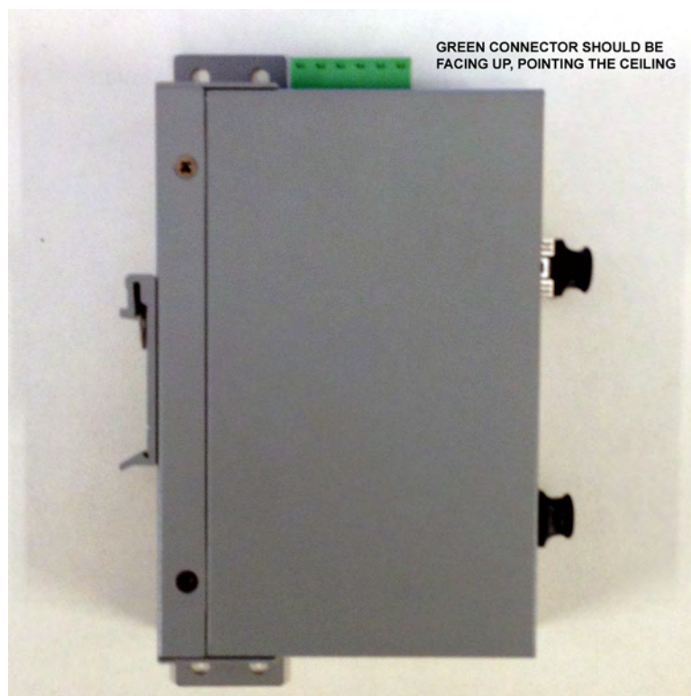
FIGURE 3-4 Wall-Mount Plate Fixing
