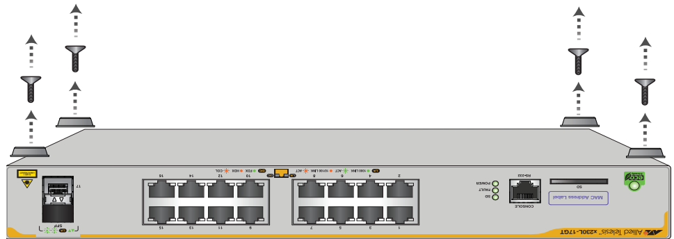
FIGURE 14. REMOVING THE RUBBER FEET FROM A SWITCH
