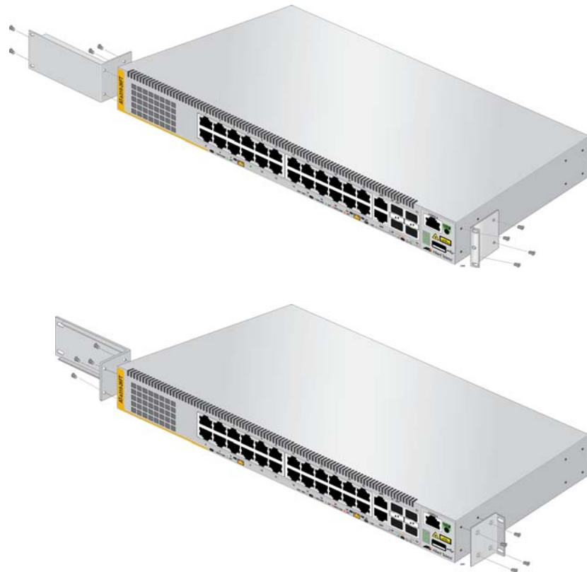
Figure 25. Installing Brackets on the AT-x310-26FT Switch
