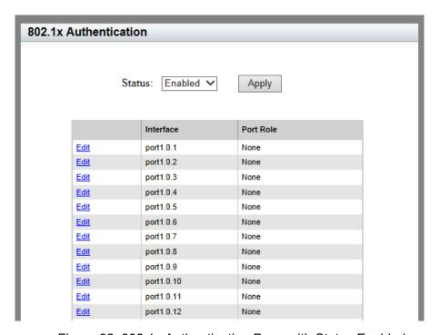
Figure 82. 802.1x Authentication Page with Status Enabled
