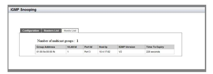
Figure 59. IGMP Snooping Page with Hosts List Tab
