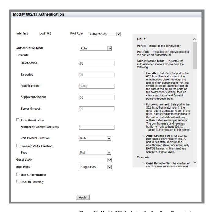
Figure 81. Modify 802.1x Authentication Page Expanded
