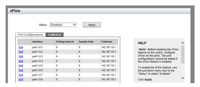
Figure 144. sFlow Page with the Port Configurations Tab
