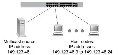
Figure 60. IGMP Snooping Querier with One Querier
