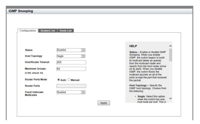
Figure 57. IGMP Snooping Page with Configuration Tab
