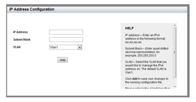
Figure 85. IP Address Configuration Page
