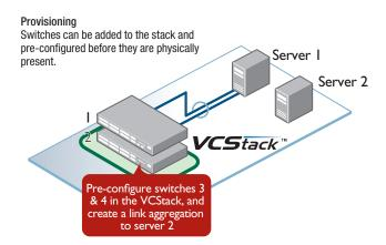
Switches 3 and 4 are automatically configured when they are connected.
