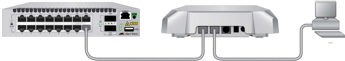
Figure 23. LAN2 Port in Cascade Mode with an End Node
