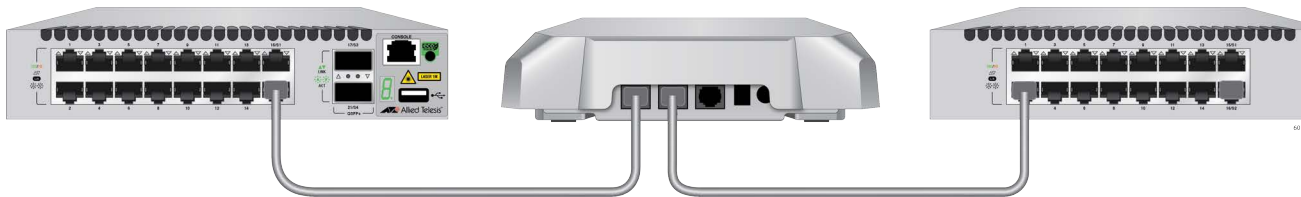
Figure 24. LAN2 Port in Cascade Mode with a Networking Device
