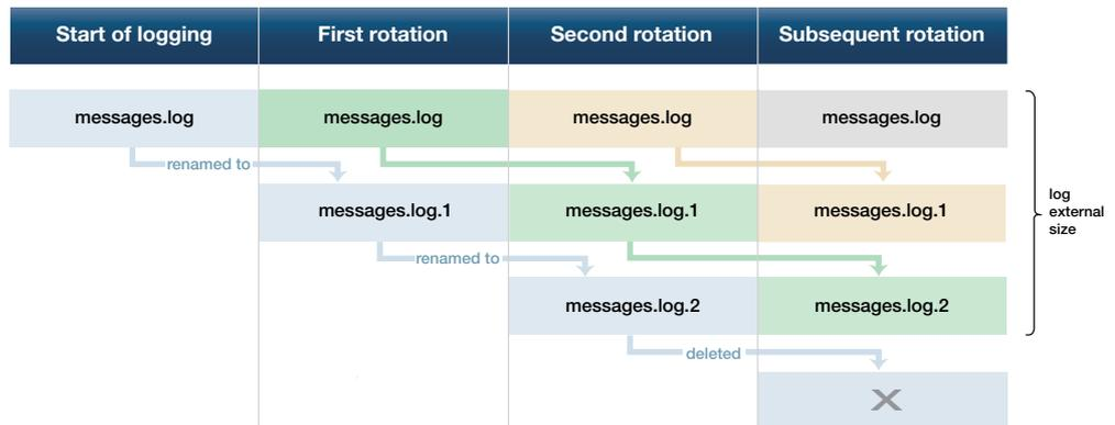
Note that if you set rotate to 0, and the external log file becomes full, then the device deletes the full log file and creates a new (empty) file of the same name to save messages into. For this reason, we recommend setting rotate to at least 1.
